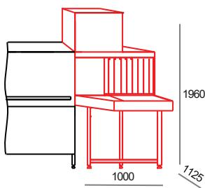
**TC90 – AS Blower Dryer on 90° exit curve without motor**
