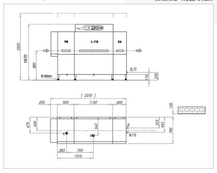
The drawing refers to the standard machine with no optional - Feeding direction: left / right
