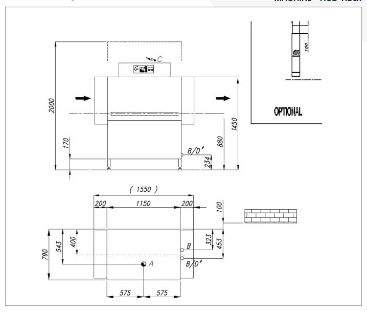
The drawing refers to the standard machine with no optional - Feeding direction: left / right
