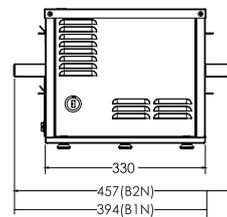
Installation requires minimum 0.25" (6mm) clearance on each end.
