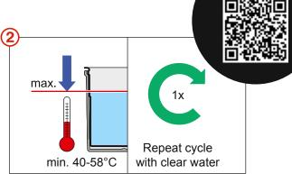
Attach the pacotizing® blade and spray guard, fill the pacotizing® beaker to the maximum fill line with 40-58 °C warm water, add a Pacojet Cleaning Tab, attach the pacotizing® beaker and protective beaker, start cleaning process.
