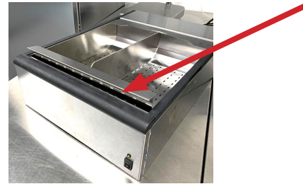
Incorrect placement of the food tray. Front edge is too high.
