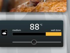
The integrated core probe's six measurement points detect product sizes and quantities, so every dish reaches the set core temperature – and the target results – precisely. The dish is prepared exactly the same way next time.
